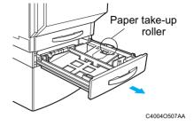
Press down on the paper-lifting plate until it locks into place.
