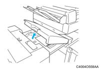
Remove any paper, and then close the cover of the horizontal transport unit.
