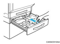
Load the paper into the drawer so that the front side of the paper (the side facing up when the package was unwrapped) faces up.
