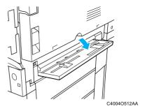
Adjust the paper guides to fit the size of paper to be loaded, and then load the paper so that the front side of the paper faces down. Lightly slide the paper into the feed slot as much as possible so that it is ready to be fed into the copier.
