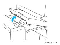
Remove any paper, and then close the cover of the horizontal transport unit.
