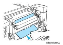
Move the two lock release levers for the oil-coating unit in the direction of the arrows.
