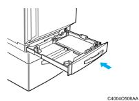
Turn the media type selection dial on the drawer to the setting for the type of paper loaded.
