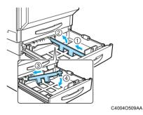
Slide the lateral guides to fit the size of paper to be loaded.
