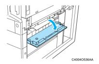
Turn the green wheels to feed the paper so that it can be easily removed.
