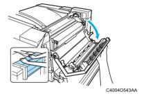
While moving the green lever on the inside of the upper right-side door in the direction of the arrow, carefully pull out the paper.
