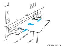
Make sure that the screen allowing you to select the manual bypass tray paper size is displayed, and then select the desired paper size.
