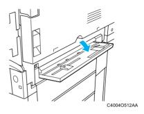
Adjust the paper guides to fit the size of paper to be loaded, and then lightly insert the paper as far as possible.
