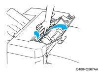
While holding misfeed clearing guide FN3 open, remove any paper.
