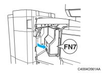
While holding open misfeed clearing guide FN8 (for finisher FN-107) or FN7 (for finisher FN-108), remove any paper.
