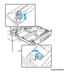
Load the paper into the drawer so that the front side of the paper (the side facing up when the package was unwrapped) faces up.
